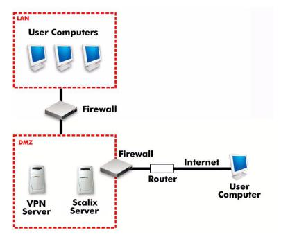
Figure 2: Scalix Installed in DMZ
