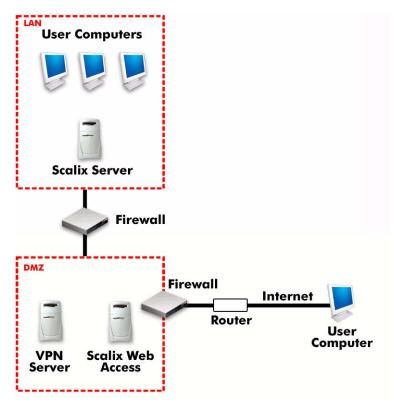
Figure 1: Multi-Server Scalix Installation in LAN and DMZ
