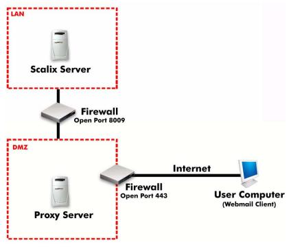
Figure 8: Apache Proxy Server as Gateway in DMZ
